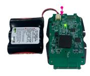
**Step 8** Connect the new the battery pack to the PCB. A green LED will flash for some seconds.
