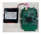
**Step 7** Disconnect the battery pack from the PCB. Be carefull in disconnecting the battery pack.
