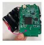
**Step 5** Lift the module and move the battery pack from the insert to the side.
