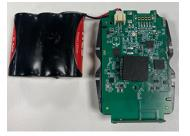
**Step 6** Align the battery pack next to the PCB and insert.
