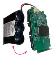
**Step 9** Move the battery pack back under the insert and PCB and flip the module.
