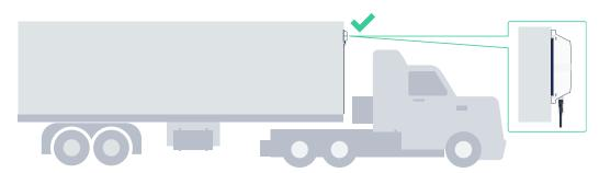
Do not install on the chassis or parts with heavy vibration.
